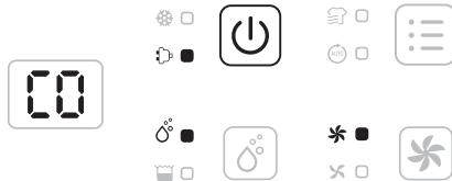
Connect the device to the mains and press the power button once to switch the device on. The device runs in manual continuous operation at high fan speed by default, and the On / Off indicator lights up.
