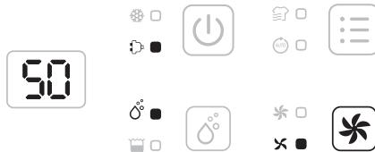
Press the fan speed button to select the desired setting (low or high).
