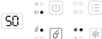
Press the Manual button to select your preferred humidity between CO-30%-35%-40%-45%-50%-55%-60%-65%-70%-80%-CO. CO means continuous dehumidification regardless of ambient humidity.
