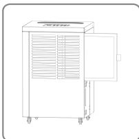
3. Remove the filter, clean the filter with a vacuum cleaner or soapy water no hotter than 40 °C.
