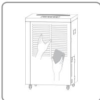
2. Clean the housing with a soft, dry cloth. If the device is extremely dirty, use a mild cleaning agent. Wipe the dehumidifier with a slightly damp cloth. Never spray the device with water.
